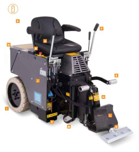
Designed specifically for high-speed soft goods removal, this machine is a durable, emission-free, budget-conscious workhorse. The 2900 will remove VCT and other soft and hard goods quickly and efficiently for time-sensitive applications.
